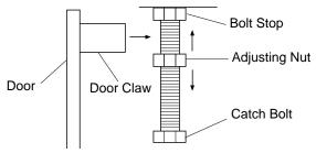
Figure 12 - Catch Bolt and Door Claw Orientation
